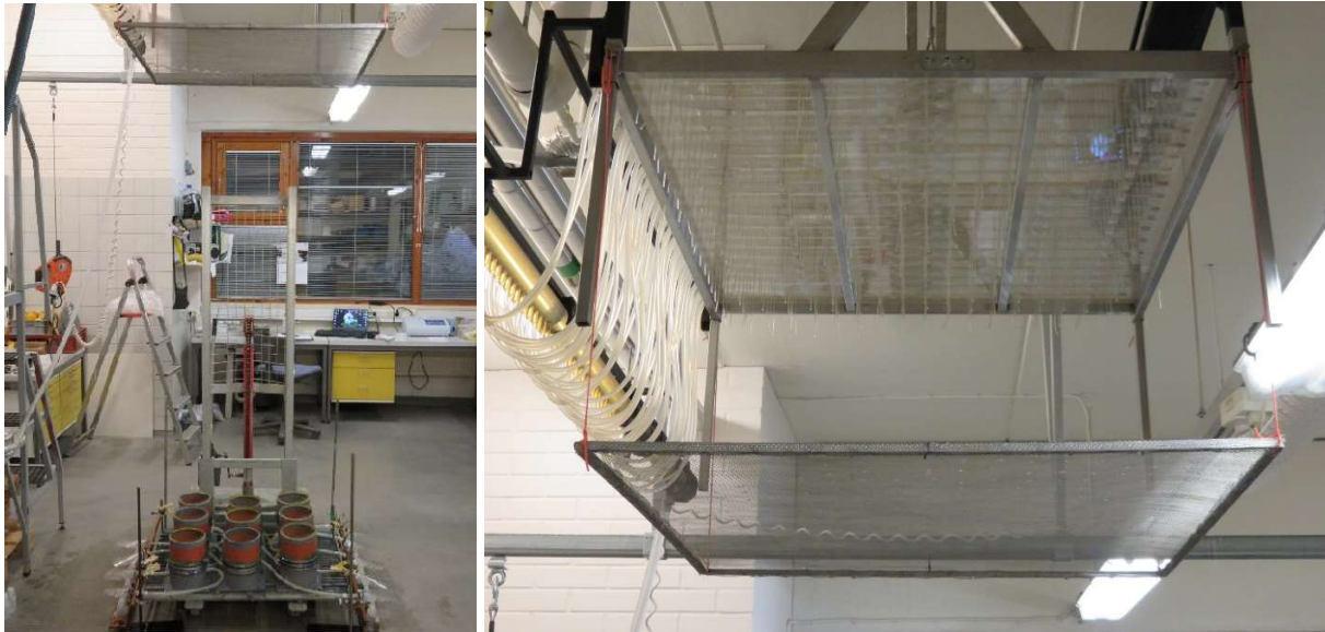
Figure 3. Set-up for the rainfall simulation. Picture on the right shows the capillars that produced rain for the simulation.
