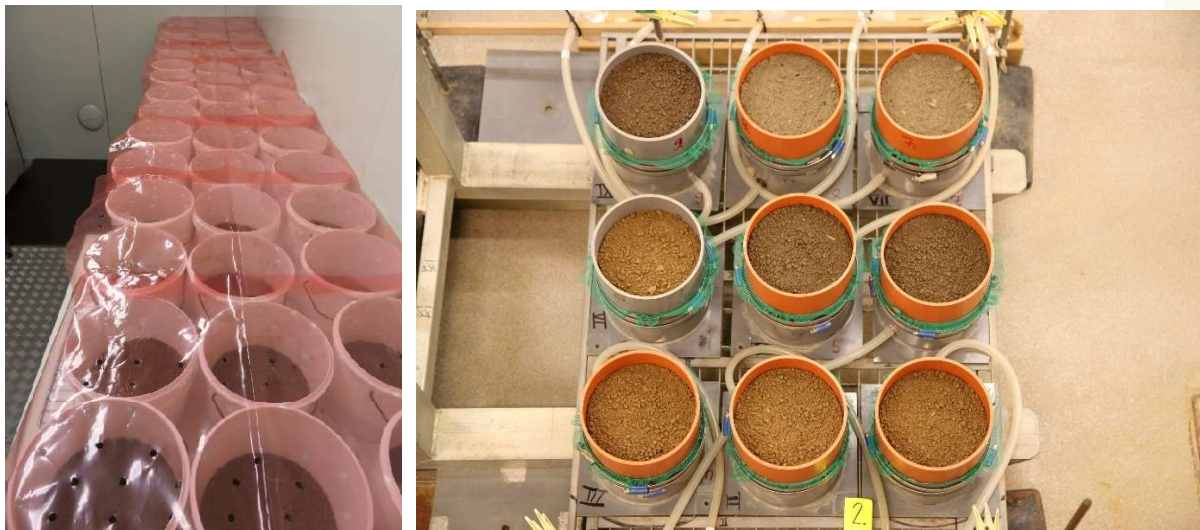
Figure 2. Incubation of soils (left) prior to rainfall simulation (right).
